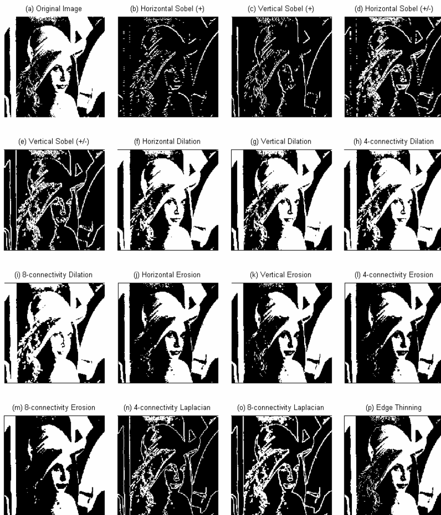
Figure 14. The outputs of 15 morphological operations on Lena image: (a) the original image, (b) – (p) the output images.
